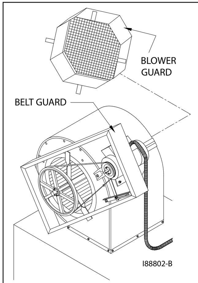
**Figure 3F - Installing the Belt and Blower Guards**
