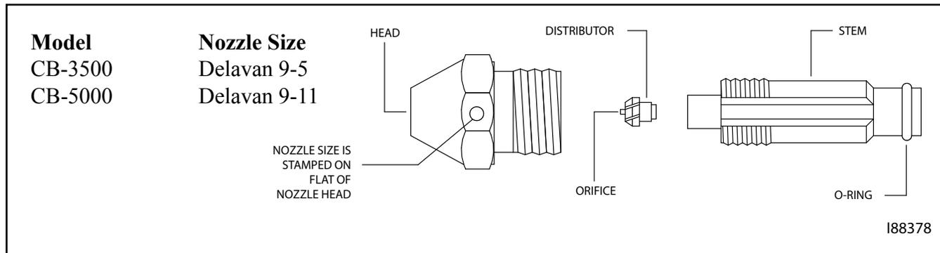
**Removing the Nozzle for Cleaning:**
