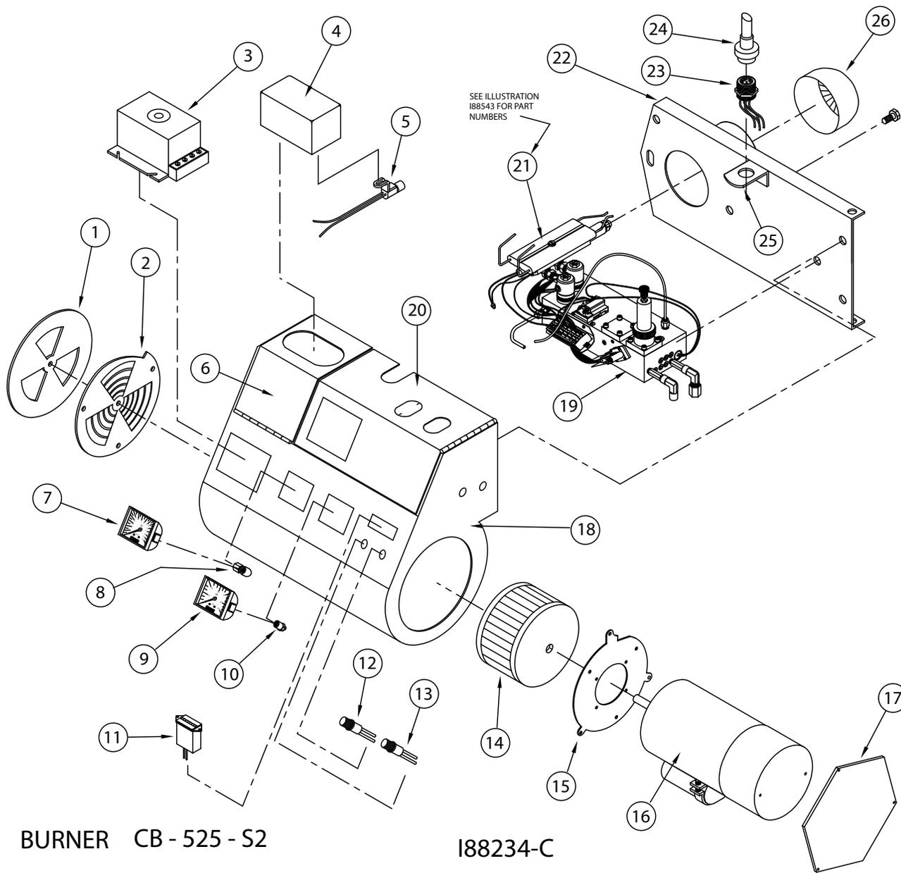
**Figure A1 - CB-525-S2 Burner Component Detail (for CB-3500 Furnaces)**
