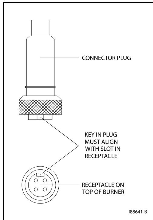
**Figure 3K - Detail of Burner Electric Receptacle**
