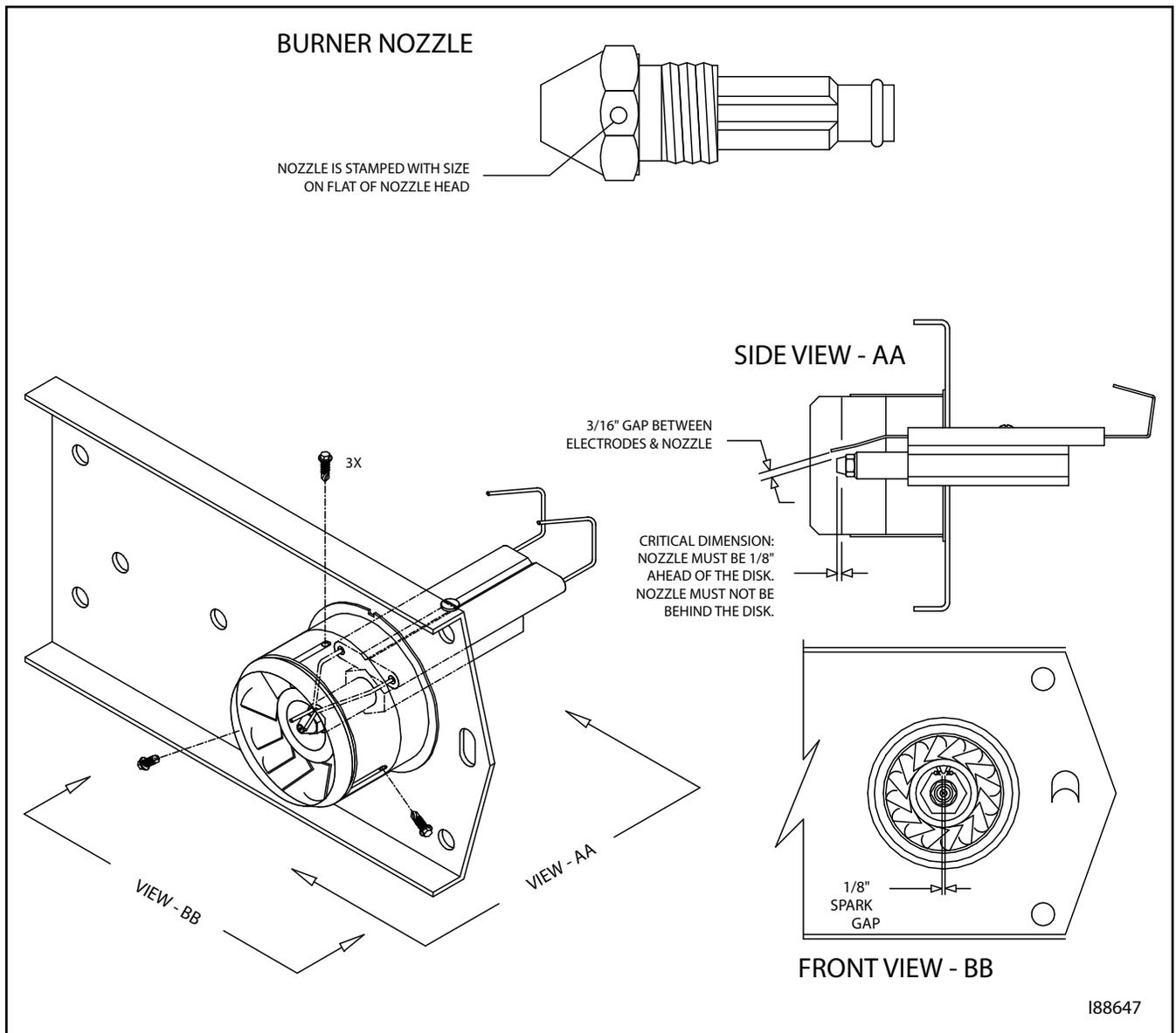
**Figure 3H - Burner Nozzle and Electrode Specifications**
