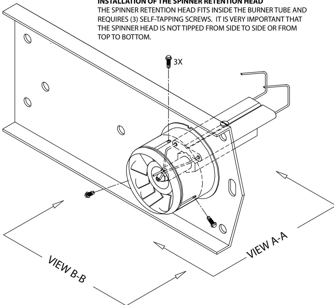
USE PROVIDED SCREWDRIVER AS WEDGE TO HOLD THE SPINNER RETENTION HEAD IN POSITION. THEN TIGHTEN THE THREE SCREWS TO LOCK THE HEAD IN POSITION.
