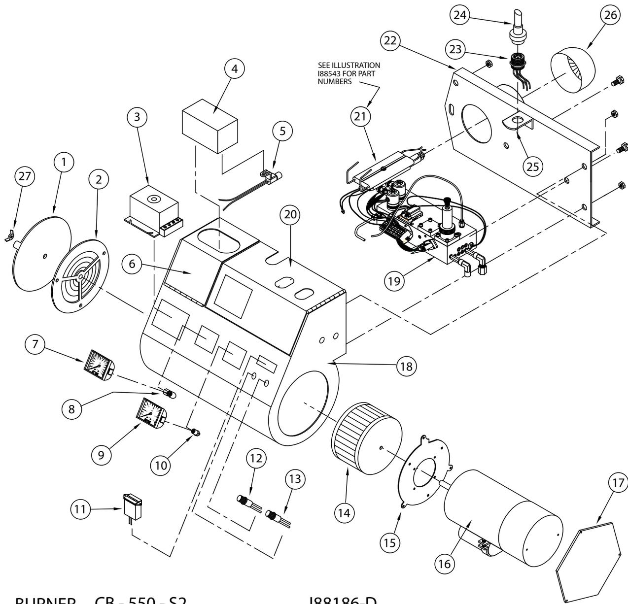
**Figure A2 - CB-550-S2 Burner Component Detail (for CB-5000 Furnaces)**
